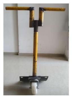
Hauler: Streamlining sack handling with an innovative carrier design. The specialised carrier stacks two 50kg sacks, reducing manual effort in loading and unloading. Hauler's ergonomic solution enhances productivity, minimises strain, and optimises logistics for handling large quantities of sacks.
